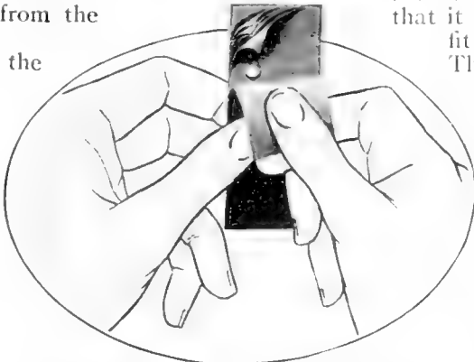
The Layers Can Be Peeled Off as Needed, the Pack Being Still Used as a Strong Solid Shim
